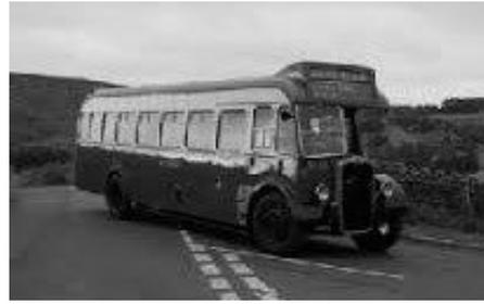
The front-engined L series Bristol single-deck bus was first introduced in 1938 but production was halted during the duration of the war. When legislation was relaxed in 1950 allowing single-deck bus to be built to a maximum length of 30feet as opposed to the previous maximum of 27ft 6ins, the LL was introduced. The new vehicle was offered with a choice of engines which were the Gardner 5LW (LL5G), the Gardner 6LW (6LLG), or Bristol's own 6 cylinder (LL6B) variant.
